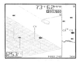
If a target is detected between the surface and the bottom and it meets the fish identification criteria, it is displayed as a fish symbol. Sonar returns that do not meet this criteria are displayed as "raw" information. Depending on the strength of the signal reflected from the target, and other factors, one of three different size fish symbols used. These reflected signals are "normalized" for depth, so that a small fish does not appear to be a large fish if it is close to the boat.
